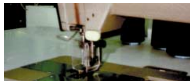
ing factory. The guard not only achieves protection of operators fingers but also protects eyes against ejection of needle particles if it shatters'
